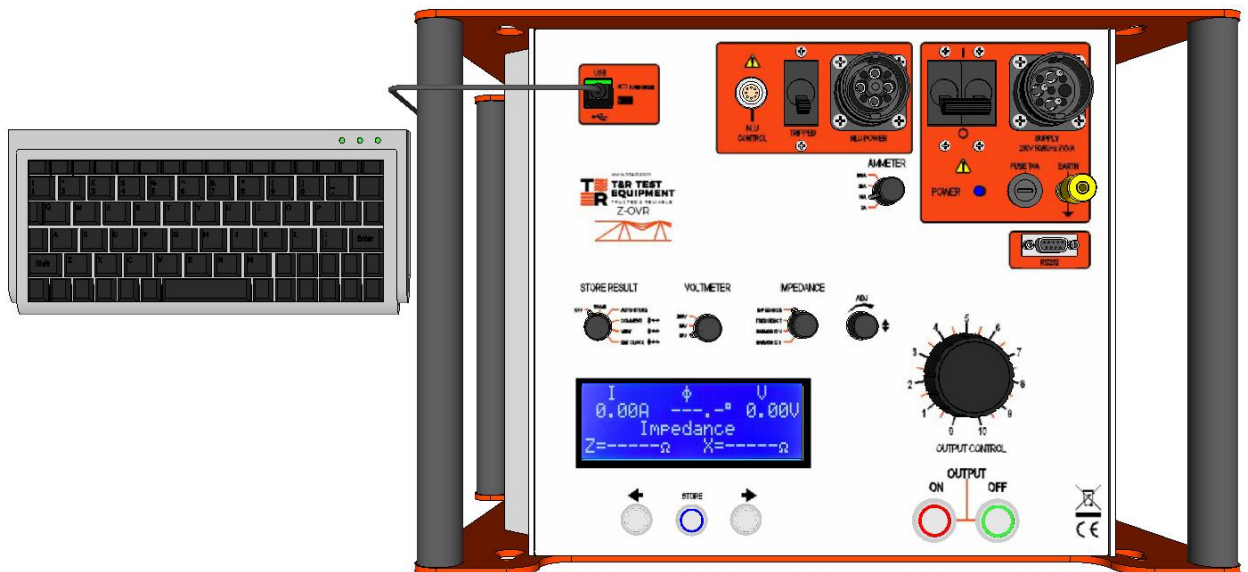
Figure 1.17 Keyboard and memory stick connected to Z-OVR (connections to output unit not shown for clarity)
